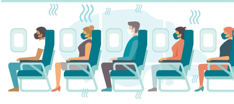
INSIDE THE CABIN, AIR FLOW FROM THE CEILING TO FLOOR, NOT FRONT TO BACK
